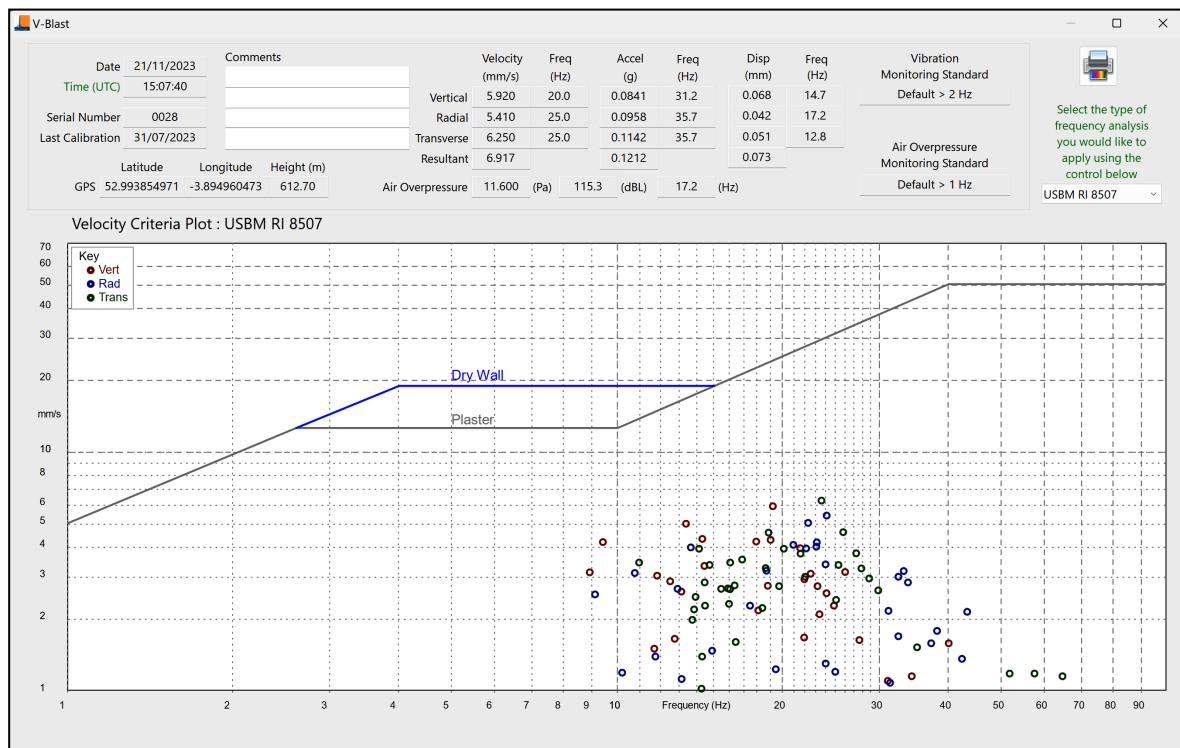
To generate a hard copy or digital output, click the **printer icon**. If a PDF printer is installed, the analysis can be exported as a PDF.
