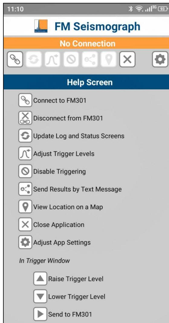
When the **FM Seismograph App** is launched, the initial screen displays a **status line** at the top of the screen, indicating the current connection state.
