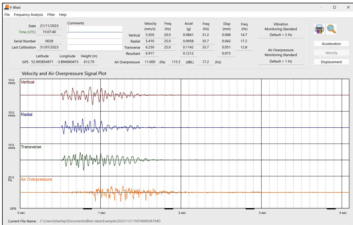
If a valid GPS signal was present during recording, **GPS time pulses** will appear along the bottom of the display.
