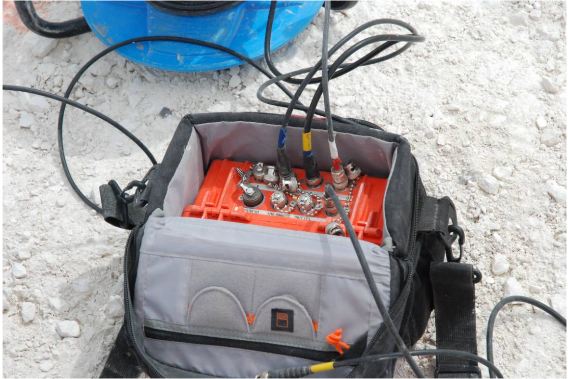
Plate 5.2. MREL Microtrap TM VOD/Data Recorder
