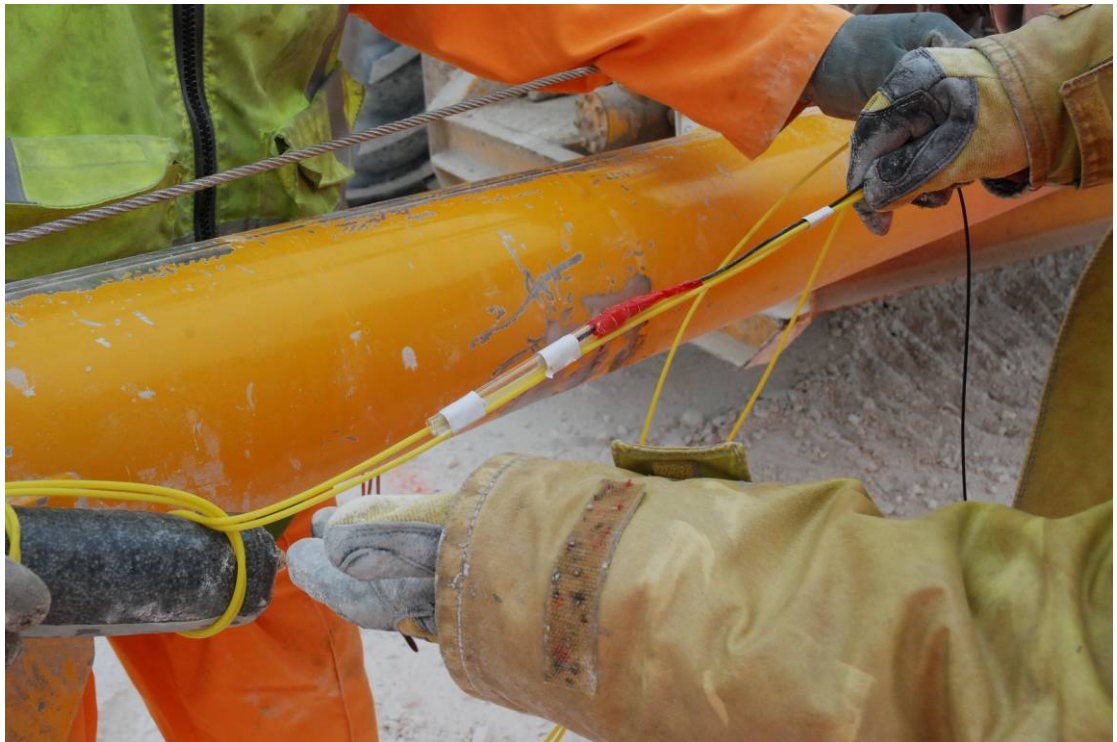
Plate 5.4 attaching Glass tubing with Optic fibre Cable to down hole Shock Tube
