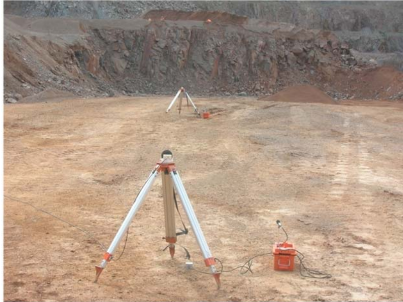
Plate 4.4 Air overpressure microphones positioned directly in front of the first blast hole
