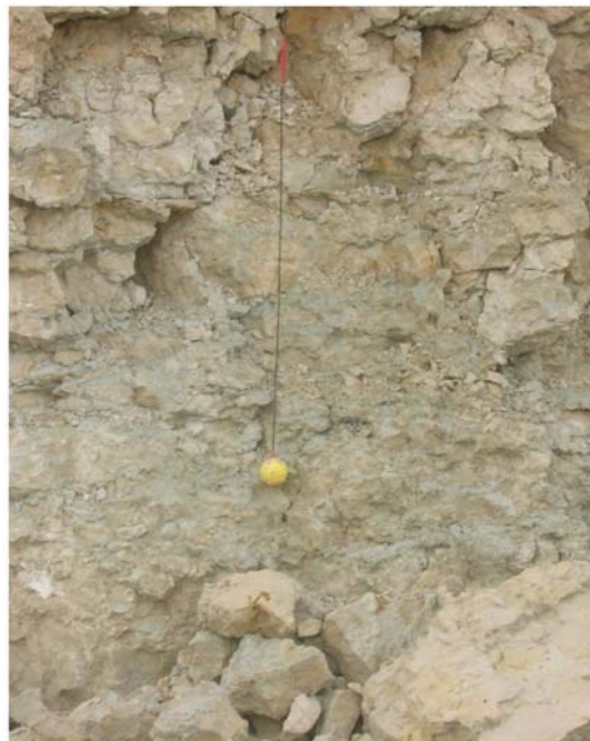
Plate 4.3 Face sensor is encased in a rubber ball, positioned in front of the face
