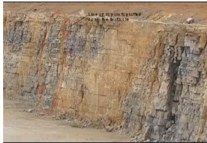
Figure 3.3 Inserting points to monitor face velocities from a particular hole.
