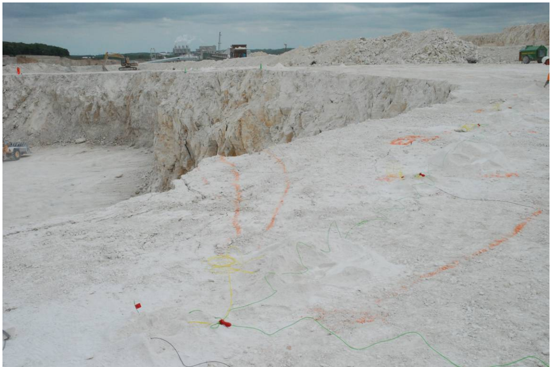
Plate 5.5. Lowering primer cartridge with Shock tube detonators and Optic fibre cable down the blast hole
