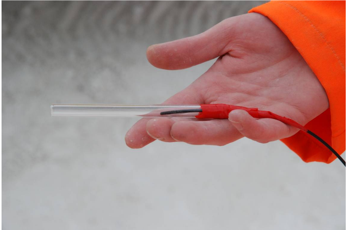
Plate 5.3 10 mm (0.4 in) diameter x 10 cm (3.9 in) length of laboratory glass tubing with Optic Fibre Cable
